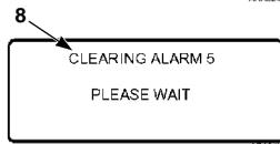
8. After the alarm situation is resolved press the Clear key to clear the alarm. To display the next alarm, press the Next key.
